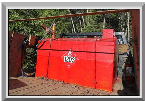
Figure 25.28 Red Tidy Tank, for Gasoline.
