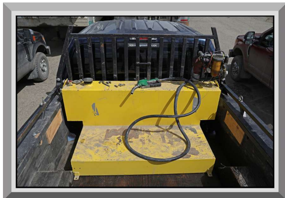
Figure 25.29 Yellow Tidy Tank, for Diesel.
