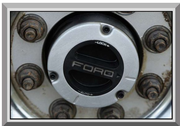
Figure 25.22 Locking Hub with "Lock" and "Auto" Options.
