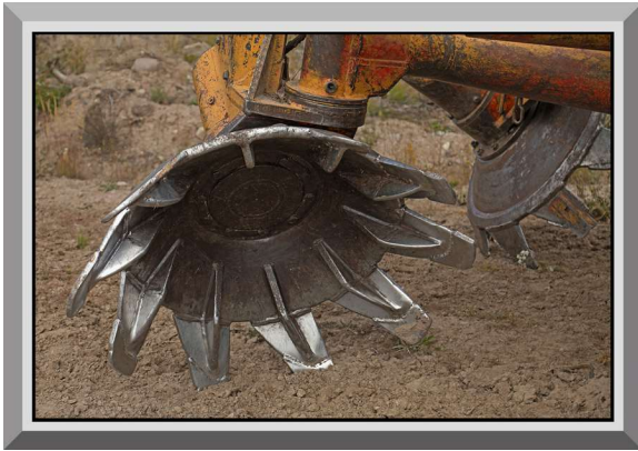
Figure 19.06 Close-Up of the Trenching Discs.
