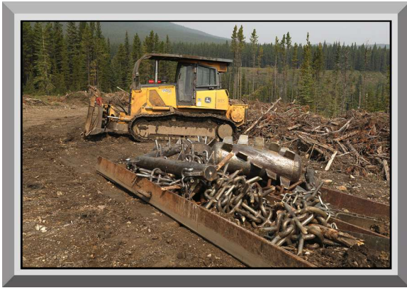
Figure 19.29 Chain Drag Machinery.
