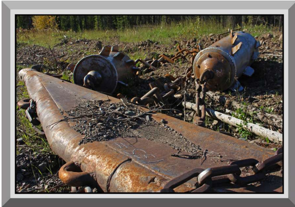
Figure 19.30 Chain Drag Attachments.
