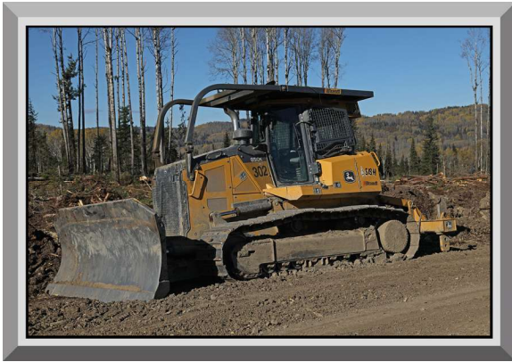
Figure 19.08 Bulldozer for Ripping.
