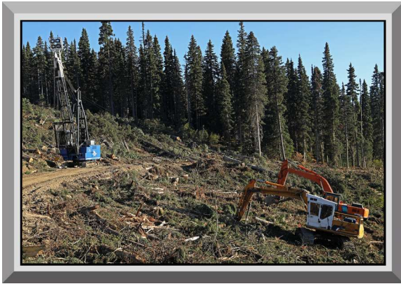
Figure 27.06 Yarder, Anchored on a Slope.
