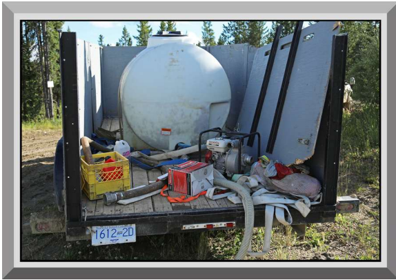
Figure 3.63 Water Trailer with Reservoir & Pump.
